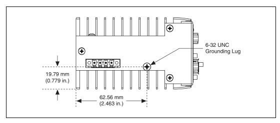
Figure C-3. Bottom View of the CVS-1450 Series with Dimensions
